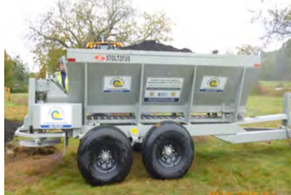
Wood Ash/ Lime Spreader: Assists in changing the pH of your soil to increase availability of nutrients.
