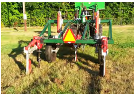
Yeoman's plow: Assists in deep subsoil compaction with minimal impacts on soil structure—and improves water infiltration.
