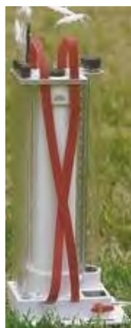
NEW! Amoozometer: Measures the in-field flow of water into a saturated soil and can be used to find actual K_{sat} values for NHDES Alteration of Terrain permits in place of book values.
