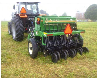
No-till Drill and Seeder: Assists with seeding without disturbing the soil.
